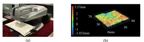
Fig. 3 – Measurement of the surface roughness: (a) measured apparatus, (b) measured surface
