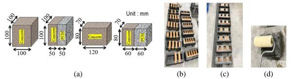
Fig. 2 – Preparation of the specimens in the experiment: (a) specimen sizes, (b) molds for the substrate concrete, (c) molds for overlaid PCM, and (d) application of the surface penetrant
