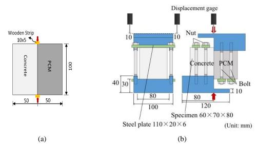
Fig. 1 – Schematic of (a) splitting tensile test and (b) direct single-surface shear test
