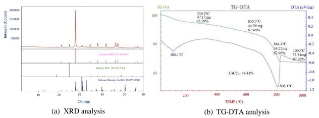
Fig. 10 - Results of X-rays analysis of powdery white compound
