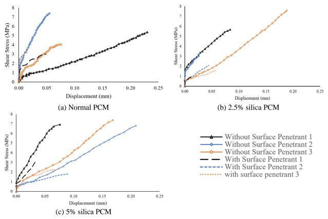
Fig. 5 - Relationship between shear stress and displacement on composite specimens
