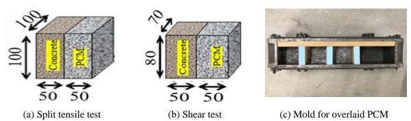
Fig. 11 – Specimen sizes (unit: mm) and mold in the reaction speed experiment
