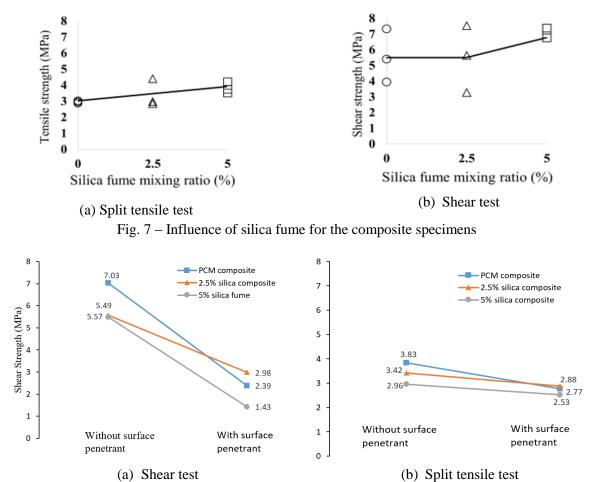
Fig. 8 – Influence of surface penetrant for the composite specimen
