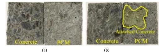
Fig. 4 – Fracture modes of the specimen: (a) interfacial fracture (I), (b) composite fracture (I-P)
