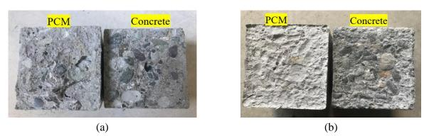
Fig. 9 – White compound at the interface of the composite specimen: (a) normal concrete-PCM composite, (b) concrete-PCM composite with surface penetrant
